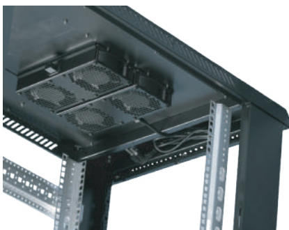
Inside view after fan module installation
