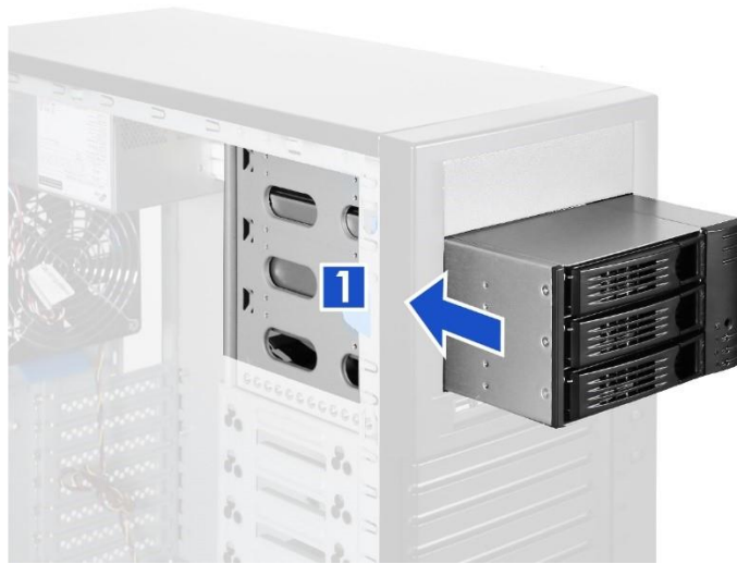
Figure 5 Storage kit installation-1
