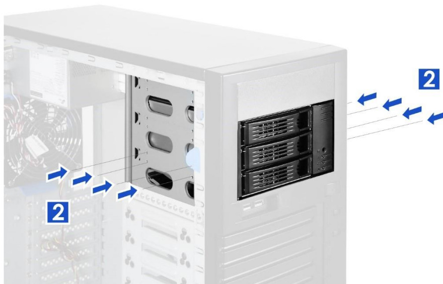
Figure 6 Storage kit installation-2
